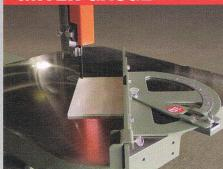
Cut precision miters with this attachment. Indexable from 0° to 45°.
