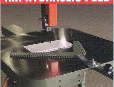
Enables operator to manually direct workpieces as they are fed into the saw blade.
