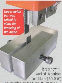
was installed on the Grob 4V-18 Band Saw. This installed blade was restrained in a torque test fixture. Then, the guide bar secured the test fixture against the saw table. The Band Saw was energized... and the blade failed.
